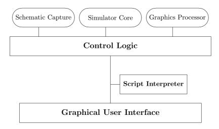
Figure 1.1: Block diagram of the WRspice interactive circuit simulation tool.
